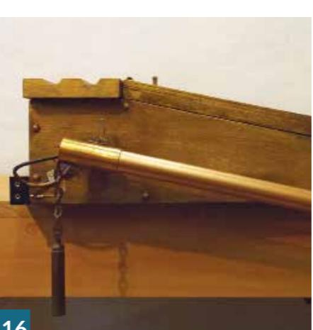
**16** The completed light assembly. A counterweight and a small safety chain were added to avoid causing unnecessary strain on the mechanism.
