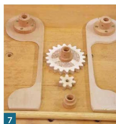
**8** The sides were drilled with a 15.875mm Forstner bit, to allow movement of the axle without too much play. As part of the decorative aspect, the heads were cut from some steel rivets. These would be glued into holes drilled in the panels to give a more industrial effect.
