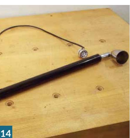
**14** An LED cluster was removed from a torch bought at the pound shop and the connecting cable soldered on. Hot melt glue was then used to insulate the back of the cluster. Part of an old light fitting and a piece of plastic pipe were assembled and sprayed to complete the unit.
