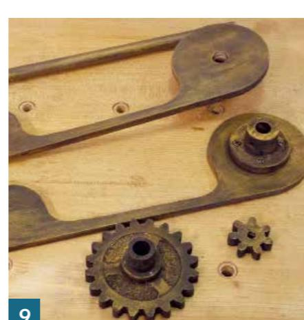
**10** The frame was sprayed with a combination of black, gold and copper paints and assembled with the mechanism installed. Gilt cream was once again added as a highlight.
