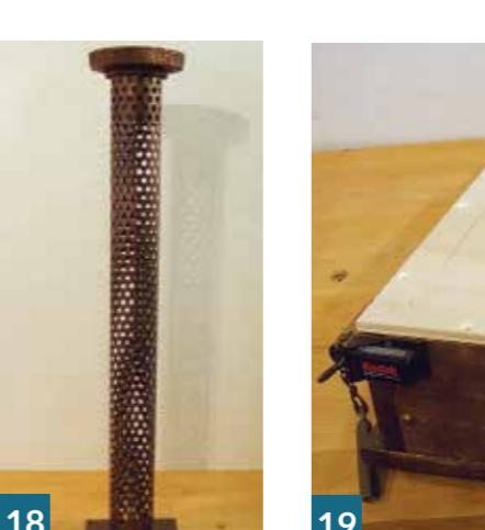
**19** Next, a piece of ply was cut for the bottom, drilled, countersunk and marked out for the central support. ▶
