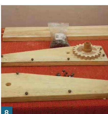
**9** All the moving parts were stained, rather than painted, to ensure wear would not expose bare wood after continued use. Gilt cream was also applied to give a more metallic effect.
