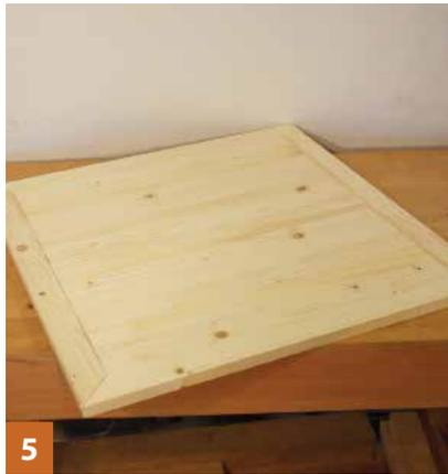
**6** Construct the top using a loose tenon arrangement, again to allow for expansion or contraction of the timber. Set the router table to create a rebate in both sides of the internal pieces and the inner sides of the mitred frame.
