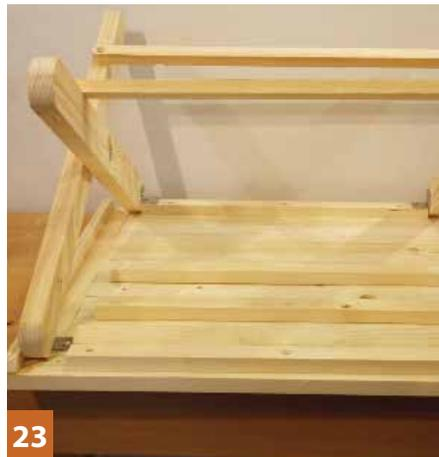
**24** Break down the table into its component parts, then sand and fill. I decided to leave it looking natural, so I finished with Danish oil. It could, however, be scorched or coloured with stain to suit.
